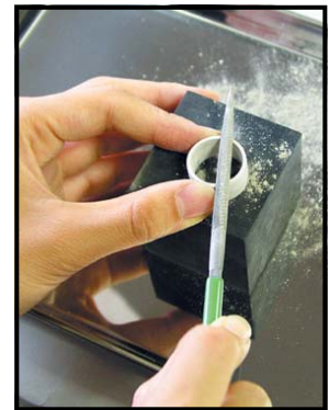
Support dry rings on a rubber block when sanding, filing and shaping
