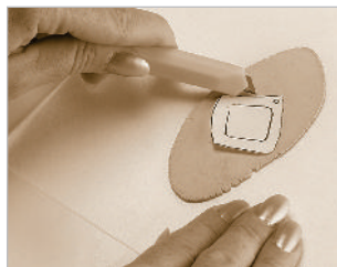
Use a sharp edge to cut BRONZclay™.
