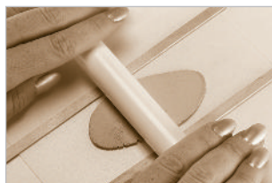
Use stirring sticks as a thickness gauge.
